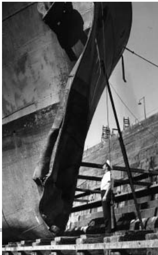
LEFT: A sailor examines the damage to the bow of the minesweeper Kiwi sustained during the attack on I-1 off Guadalcanal. OPPOSITE: U.S. intelligence personnel examine the twisted remains of the Japanese submarine I-1 after the vessel was sunk. Her hulk yielded valuable intelligence documents including the first Japanese codebooks captured by the Allies.
